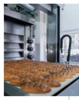
The high-capacity Vulkan Impact with the double loader Concord rapid at the exit end of the oven. The Concord rapid manages the entire batch of baked goods for an oven on 2 loaders, one above the other.
