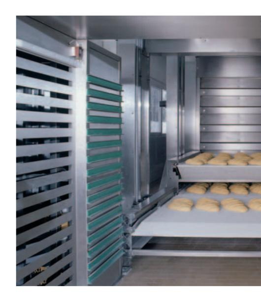
Equipped with the unique Heuft high-performance double loader Concord rapid – in double step a complete hearth can be loaded and unloaded in a matter of seconds – and all products can be baked with the Vulkan Impact – one for all, all in one.
