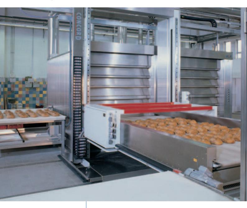
At the bakery, Mantei in Heidelberg: 2 Vulkan Thermal-oil deck ovens, each has 6 hearths, 187.5 x 240 cm, 27 sqm baking area, prepared for 9 hearths. The Concord can be moved transversely, and in expanded stage can load up to 3 ovens each with 9 hearths (121.5 sqm baking area). Each hearth group, 3 hearths with 13.5 sqm baking area, is individually regulated.
