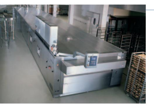
The single-hearth continuous oven at the company, Roelandt in Zele/Belgium. The oven is 205 cm wide, 2,040 cm long (41.82 sqm baking area) and has 6 temperature circuits. Baking is done continuously on wire belt in 3 shift operation.
