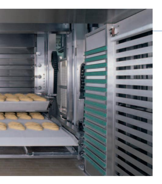
This is the high-capacity compact oven, Vulkan Impact, with the double loader Concord rapid at the bakery, Richard Nußbaumer GmbH in Waldbronn. The oven has 5 hearths, 250 cm wide, 480 cm long. Each hearth has 12 sqm baking area, the entire oven has 60 sqm overall baking area. You can reach Herr Nussbaumer under the phone number ++49 (0) 72 43 / 5 67 80.
