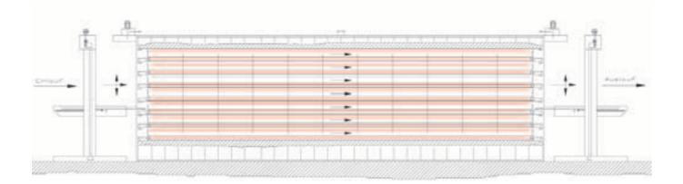
front of and behind the hearth belts and can be adjusted in height. Temperatures: Each hearth is individually controlled, mostly with separate upper and lower heating. In addition, longer ovens usually have additional temperature zones.
